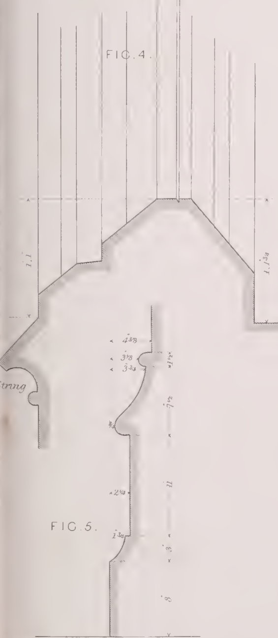
1. Plan of Mullion, Jaumb & label of Window marked B on the Elevation 2. Section thro' Sill 3. Plan & Elevation of Mullion, Jaumb of Window marked A on the Elevation 4. Section thro' Sill 5. Profile of Plinth 6. Profile of Label
